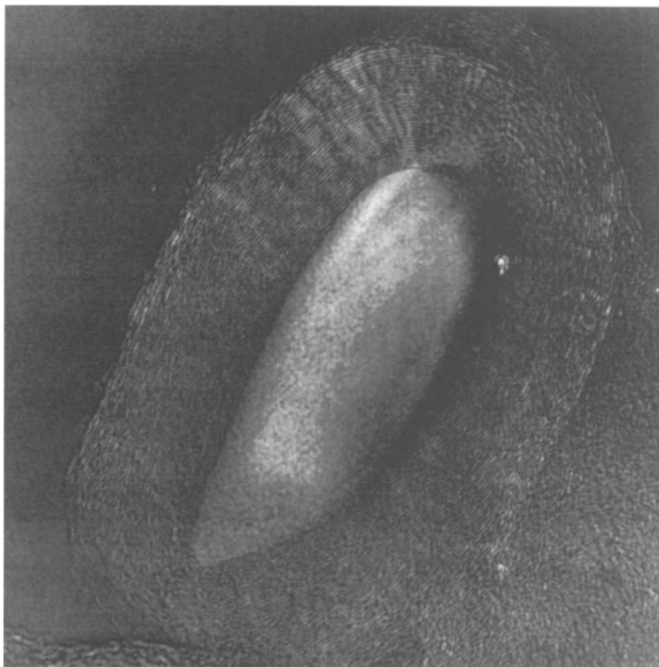
Fig. 30. Image of graphite planes encapsulating a F_3C particle with ellipsoidal shape.
